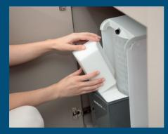
Open the lid, unwrap the block salt and place it into the tray.
