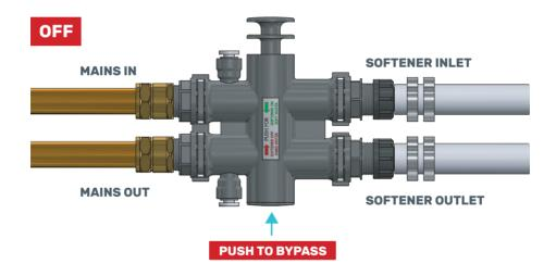
You can easily turn off your Harvey Water Softener by pushing the button in the direction of the red arrow. Each install is different, so the set up of yours might differ slightly from the diagrams.
